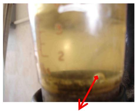
The filtration generates a few large bubbles or many barely visible bubbles through the center of the measuring tube.
