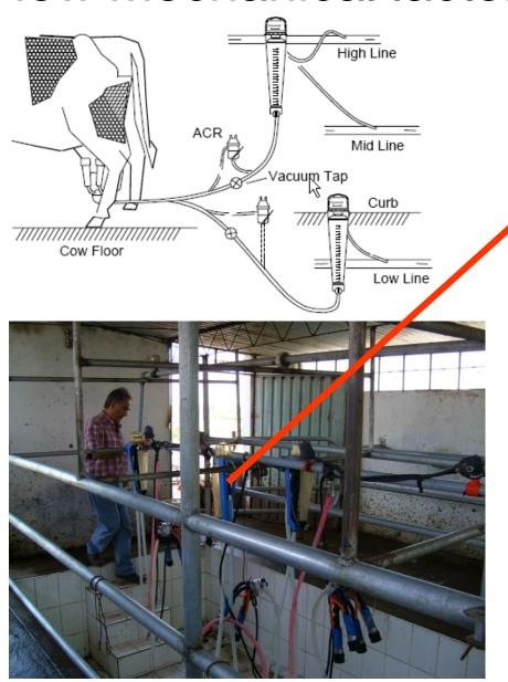
They are inserted between the collector and the milk line in each of the falls, permanently or when the control milk.
