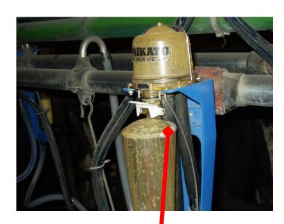
Fracture in a measuring jar fixed with glue
