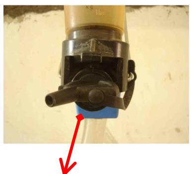
Failure in the settlement between the key and the cone housing, generally causing the light turns key filtration.
