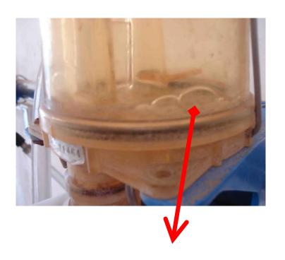
Failure in the settlement between the cover and base
