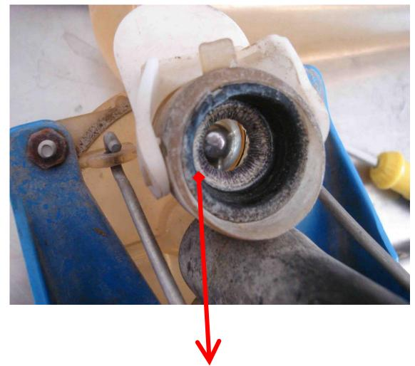
The damaged valve loses in the seat of the measuring flask.
