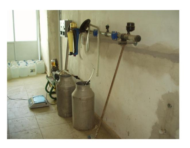
It consisted of a room, with a group of vacuum motor pump SAC, of 1.5 Hp set at 50 kPa, (15 "Hg), 20 L stainless steel vacuum and interceptor lines, dead weight type vacuum regulator, 30 L stainless steel bucket, an inlet tube, a vacuum gauge (indicates Vacuum level) and a shut-off valve .To perform the mass adjustment, a MercoCity scale, model ACS-L2 III, with a range between 0.2 - 30 Kg, and an accuracy of 0.010 Kg was available
