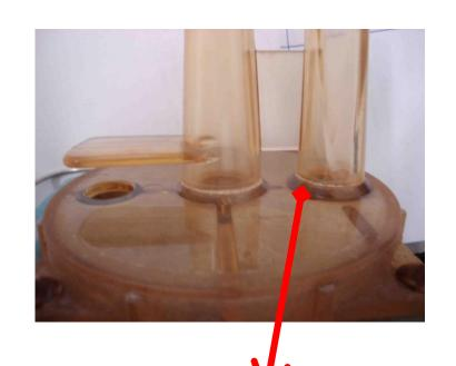
Fracture of pipe entry to the base and meter water entering the bottle
