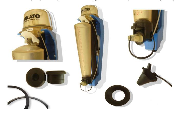
Milk meters, are basic compound instruments by at least 5 fundamental parts: cover; base; flask; 3-way valve and gaskets, which experience wear and tear continuous.
